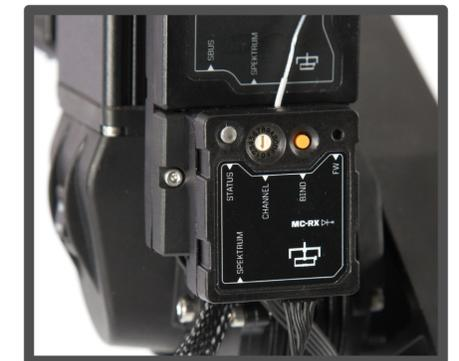
8. Attach the Receiver to the Gimbal Controller shown.
