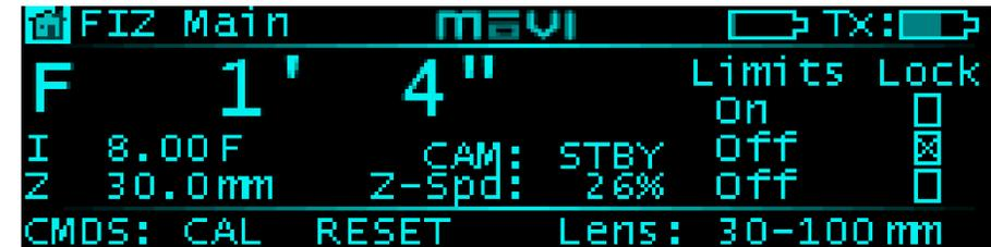
SCREEN WITH 3 AXIS LENS MAPPING ACTIVE
