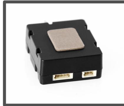
4. Remove the adhesive backing from the receiver.
