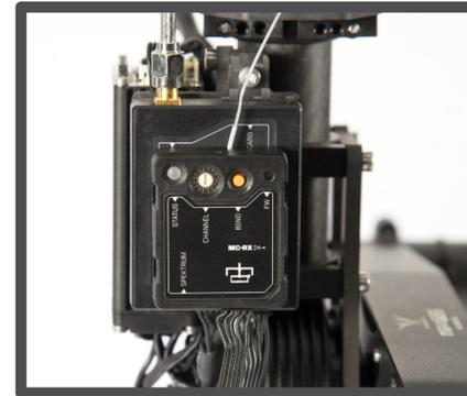
5. Attach the Receiver to the Gimbal Controller shown.
