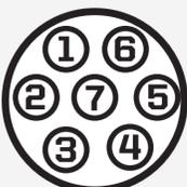
(LOOKING IN TO CONTROLLER SIDE CONNECTER) | <ul style="list-style-type: none"> <li>1 - GND</li> <li>2 - 5V Output, 1A max.</li> <li>3 - GPIO1 (0.0V - 3.3V)</li> <li>4 - GPIO2 (0.0V - 3.3V)</li> <li>5 - GPIO3 (0.0V - 3.3V)</li> <li>6 - Auxillary Data Out (3.3V digital output)</li> <li>7 - Auxillary Data In (3.3V digital input, 5V tolerant)</li> </ul> |
