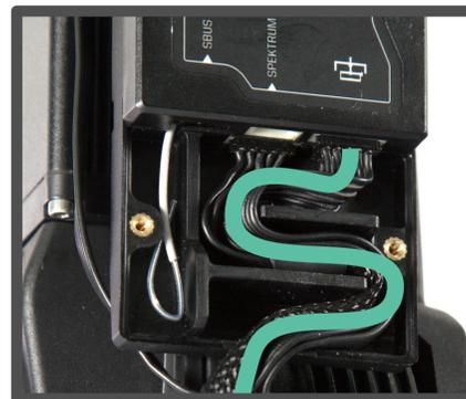
4. Route the 5-pin cable with the other wires through the Strain Relief track.
